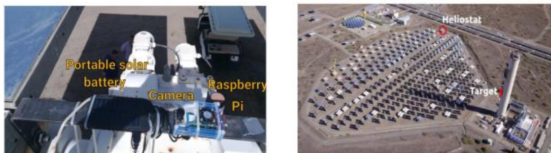
Figure 3. Smart Solar tracker prototype and selected installation in the CESA-I heliostat field (PSA).
