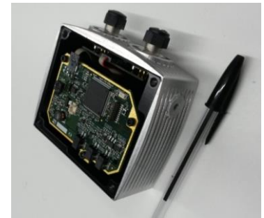
Figure 17. Internal view of the prototypes with the processing electronics in the fore front
