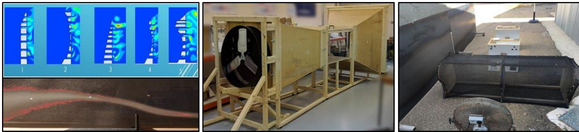
Figure 13. CFD results (top left), wind tunnel experiments (bottom left and centre) and outdoor PSA tests (right)
