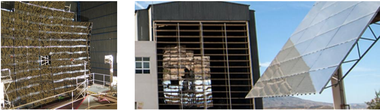
Figure 14: SF60 solar furnace; Detail view of the secondary concentrator and the OVAR test loop (left); outside view and heliostat (right)
