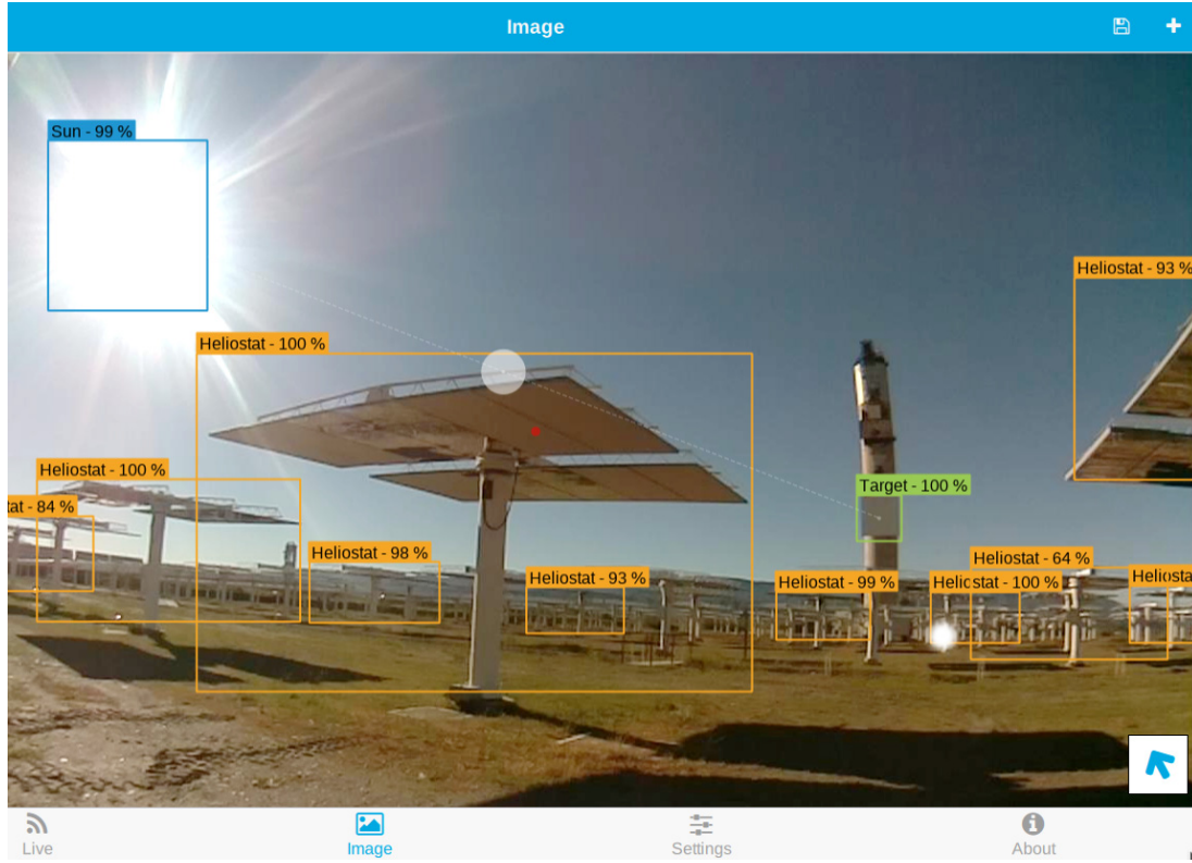
FIGURE 6. Augmented reality image processed on a mobile device at CESA solar field
