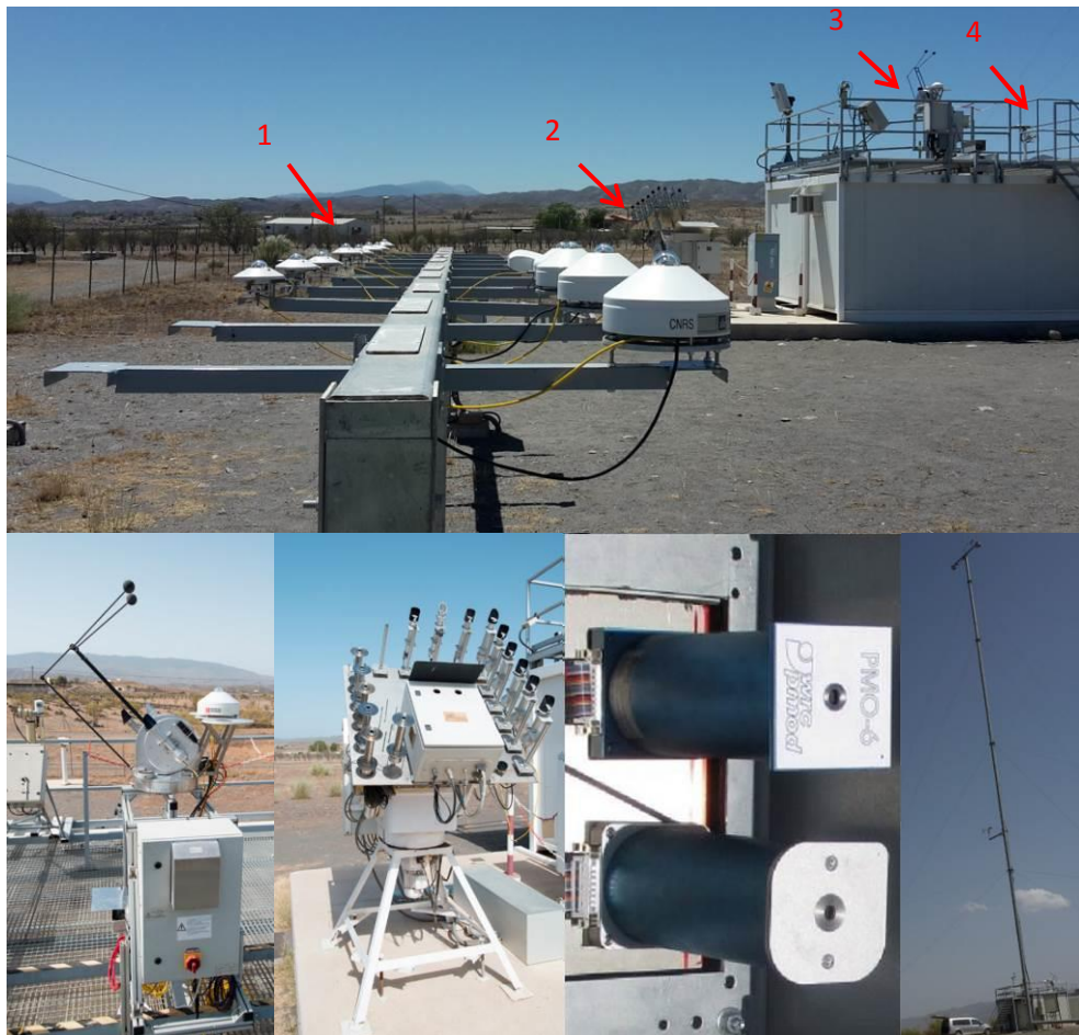
Figure 13. Top: Overview of Metas calibration setup (1: Pyranometer test bench; 2: Pyrheliometers test bench; 3: Black Photon tracker with DHI reference; 4: cloud camera); Bottom left: detail view of Black Photon tracker; Bottom left centre: detail view of pyrheliometer test bench; Bottom right centre: two absolute cavity reference pyrheliometers located in the pyrheliometer test bench's front cabinet; Bottom right: Metas wind mast.
