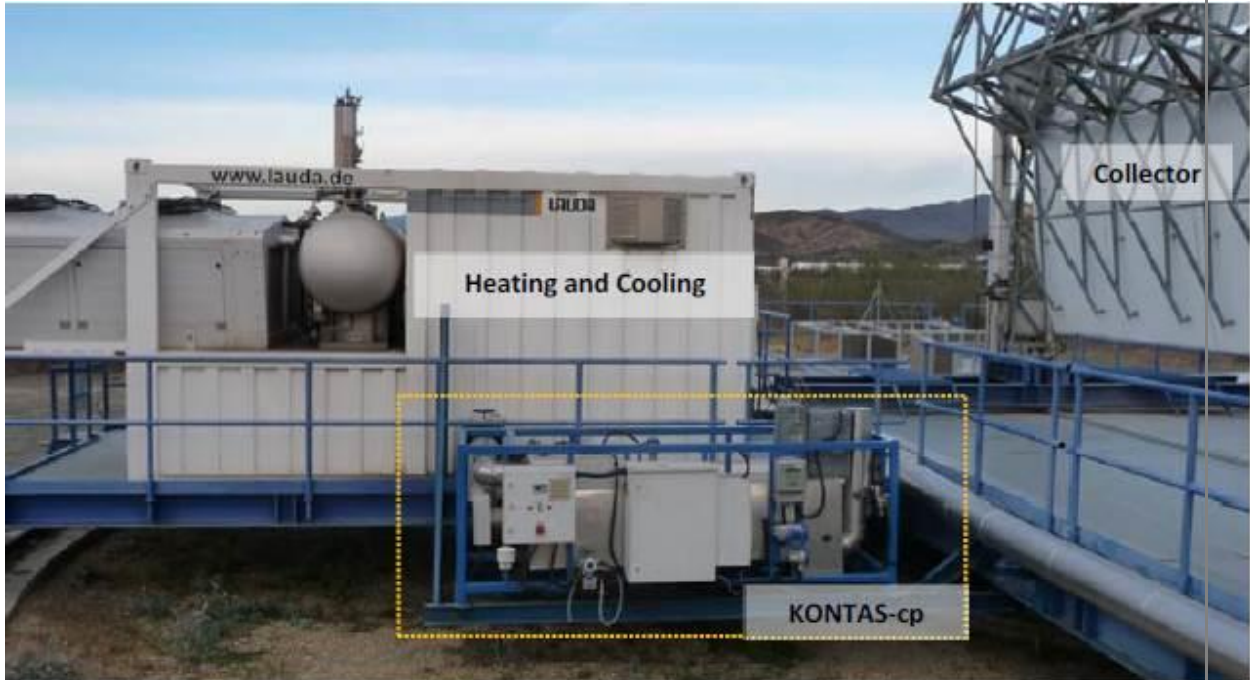
Figure 14. Calibration facility (here called “KONTAS-cp”) connected to the KONTAS facility.
