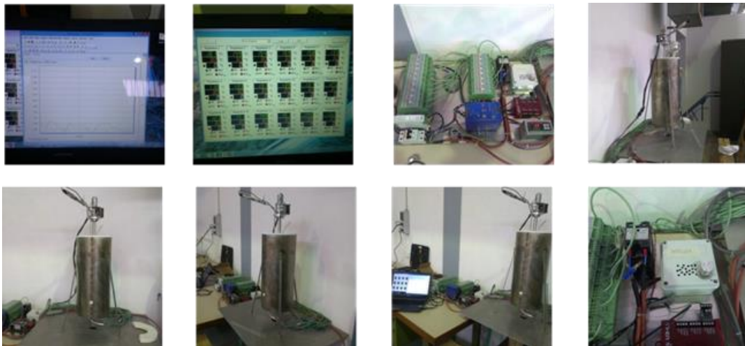
Figure 34. The experimental rig assembled at ENEA laboratories for the measurement molten salts thermal stability.
