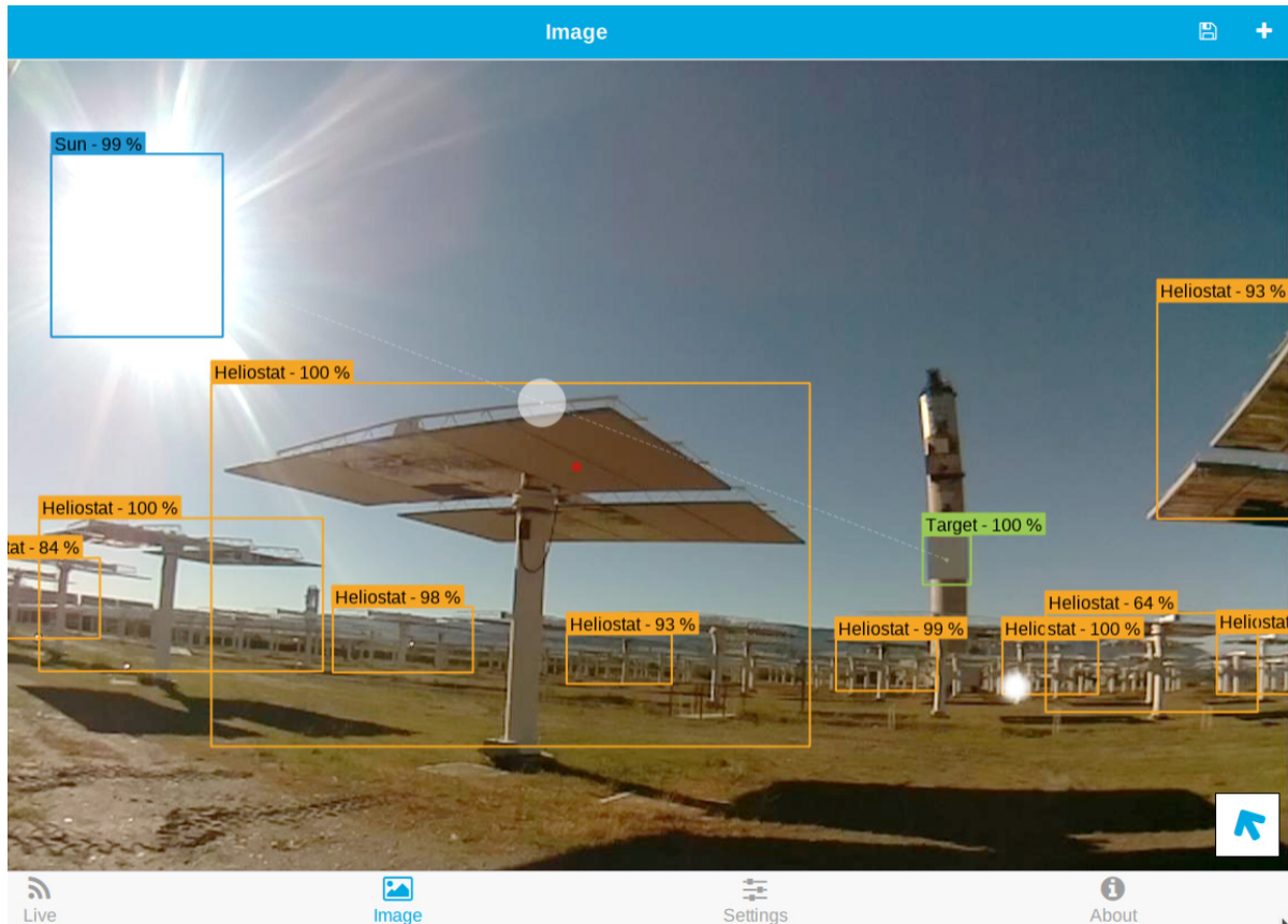
FIGURE 6. Augmented reality image processed on a mobile device at CESA solar field
