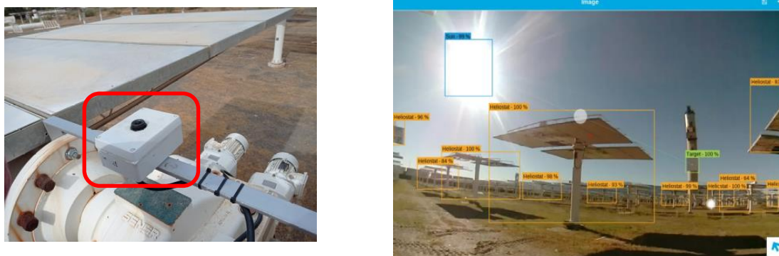
Fig. 1. Camera and embedded processor installed on a CESA I heliostat at PSA (left), and example of object recognition in recorded images (right).
