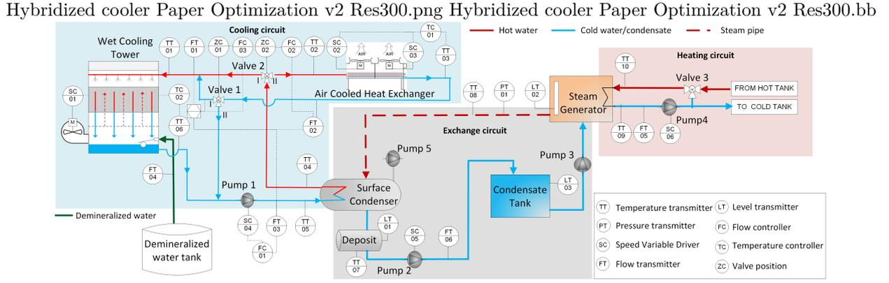
Fig. 1. Layout of the combined cooling pilot plant at PSA
