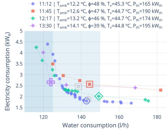
Fig. 4. Pareto fronts with the selected optimum highlighted
