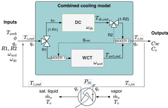
Fig. 3. Complete system model diagram
